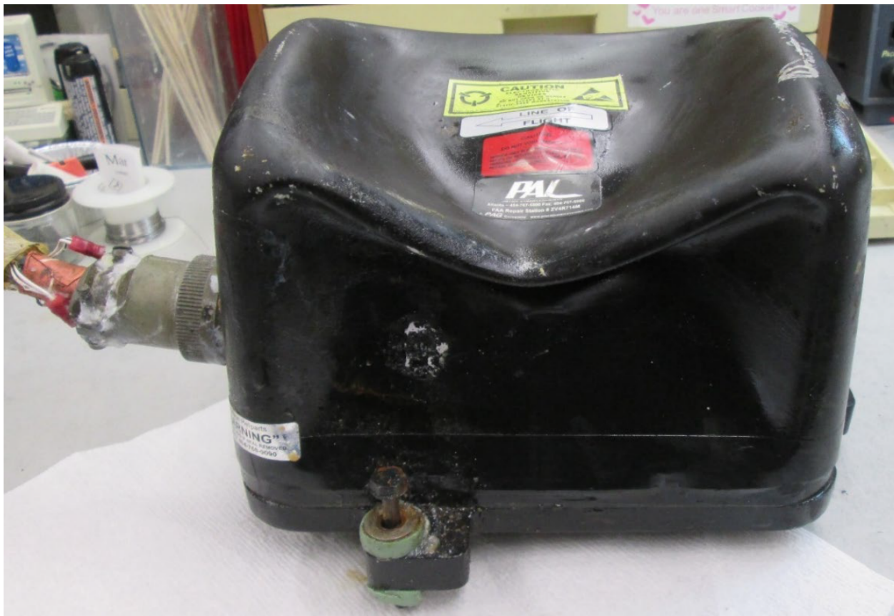
Figure 6. View of inward crushing on the vertical gyro housing.
