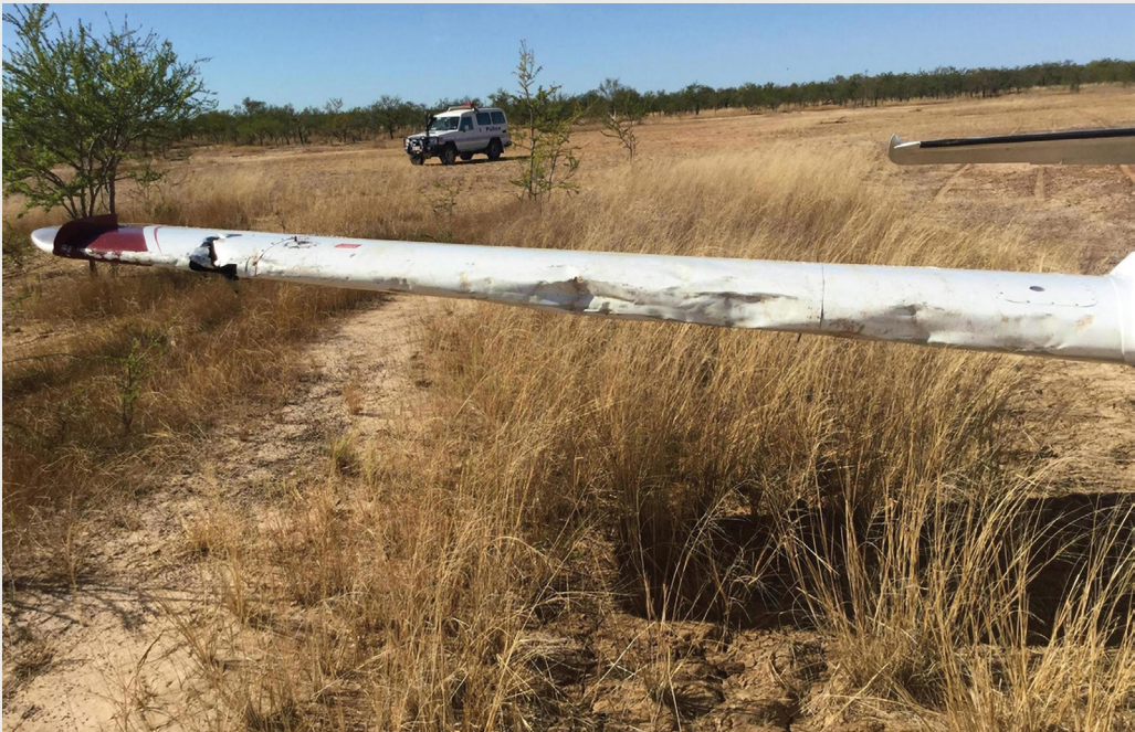
image: Damage to right wing of VH-PBU following accident © Queensland Police Service
