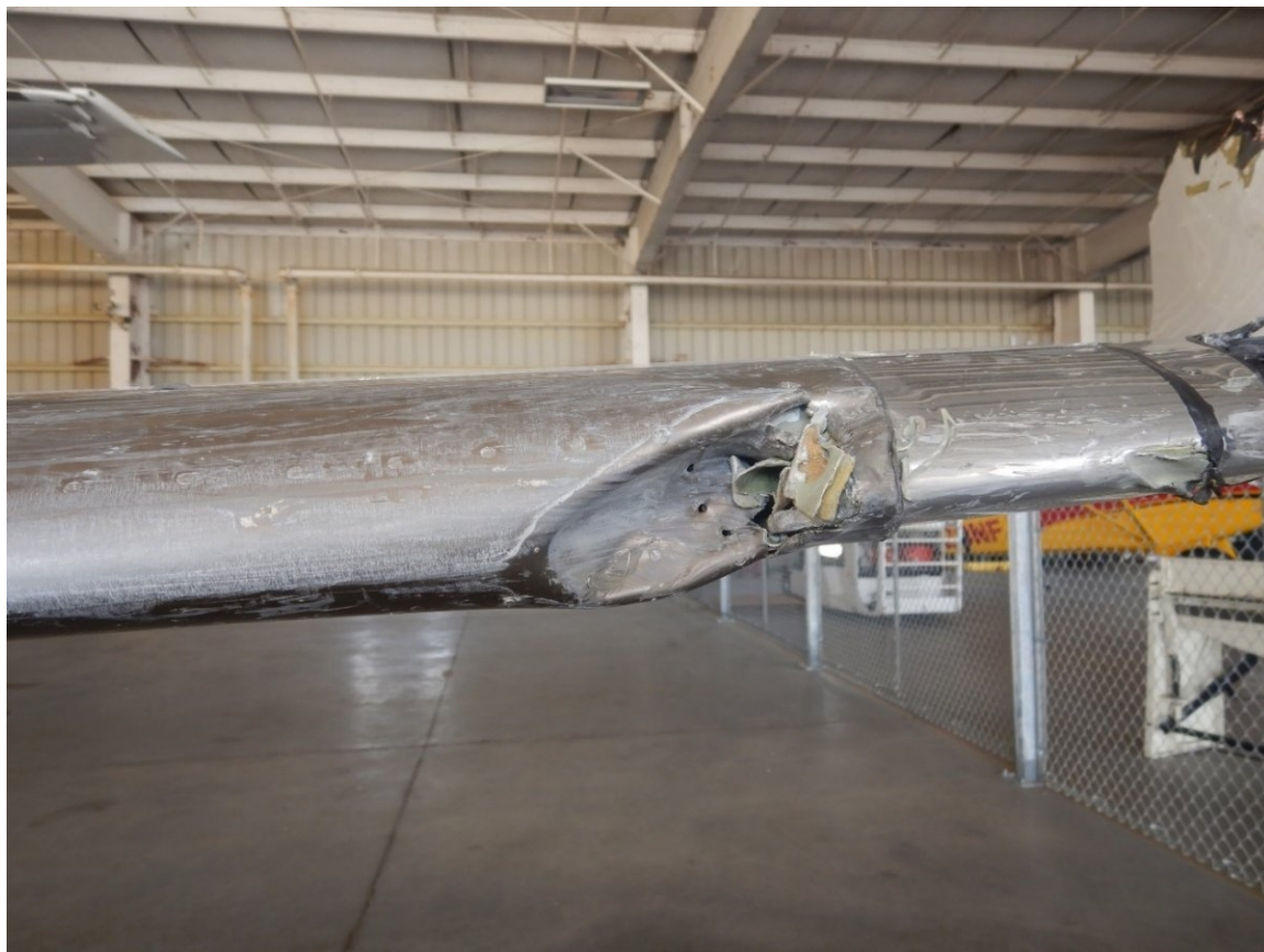
Figure 2. Close up view of N269AA's left-wing leading-edge damage.
