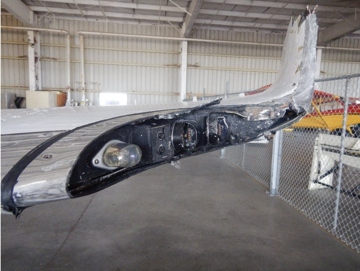
Figure 3. Close up view of N269AA's left winglet/navigation light assembly damage.
