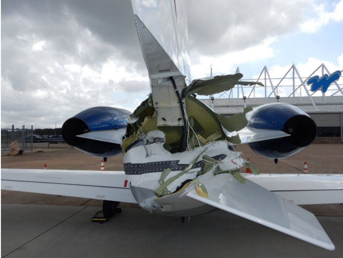
Figure 5. Aft view of N510HM's damage to its empennage.
