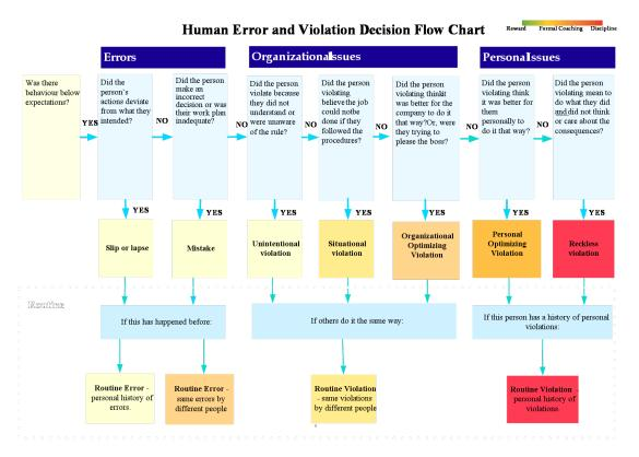
Figure 3 The decision tree for determining the types or error or non-compliance
